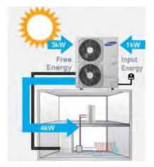
An air source heat pump works on the same principles, taking heat from the air and boosting it to a higher temperature using a heat pump.
